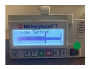
If the pump stops the light will turn red and the pump will bleep or alarm.
